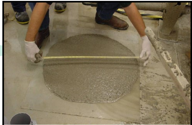
Measuring Slump Flow of SCC
