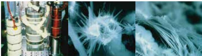
Ettringite crystals and calcium hydroxide platelet images from concrete research in zero gravity was done aboard the space shuttle Endeavour – Mission STS 68.
